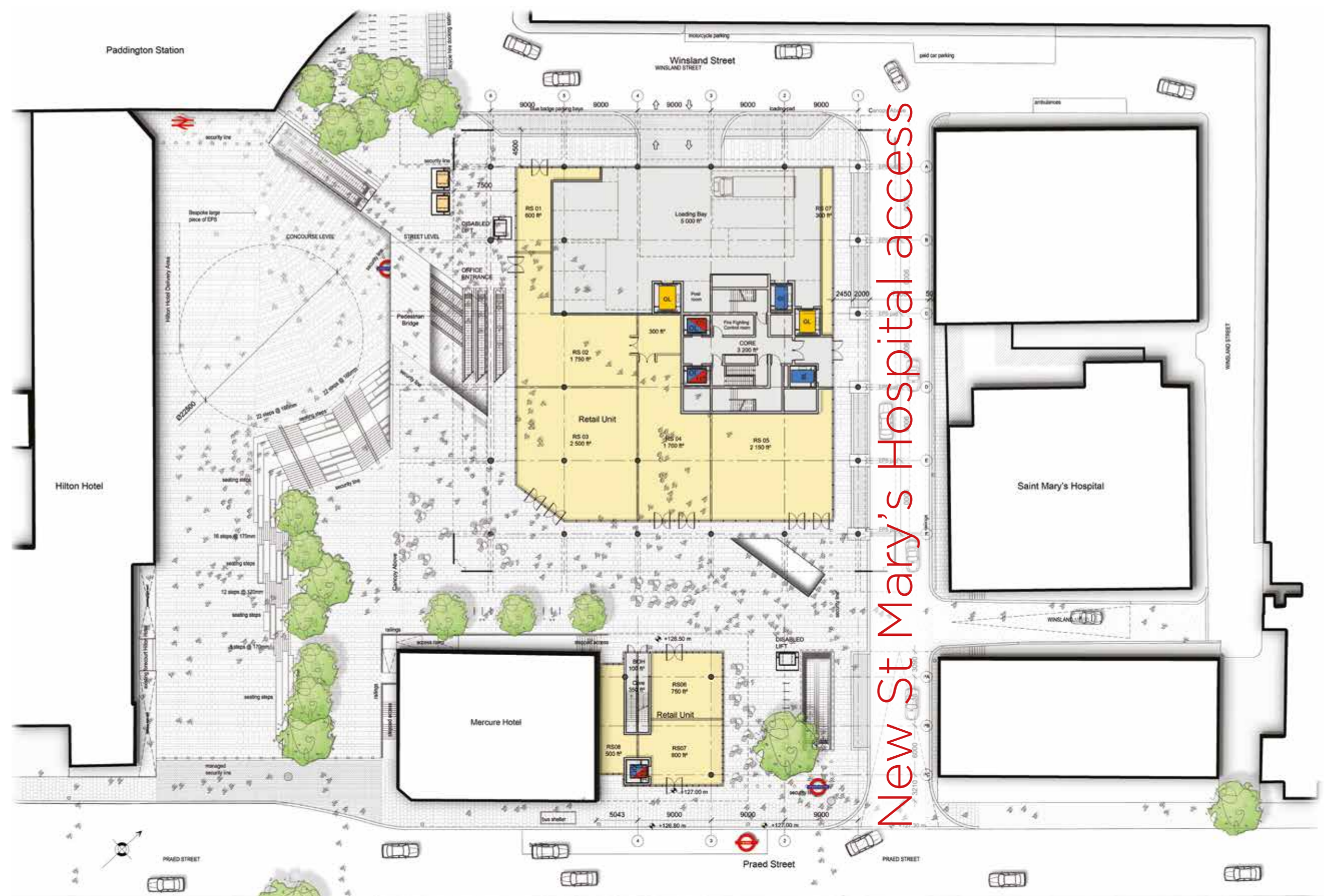
New access road for servicing and hospital access
